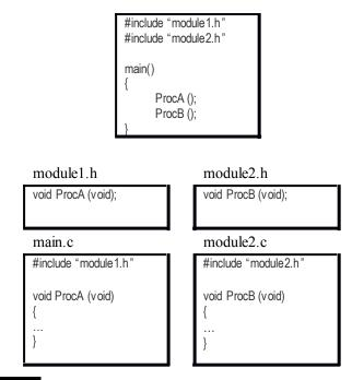
FIGURE 10-2 Program divided into separate modules
