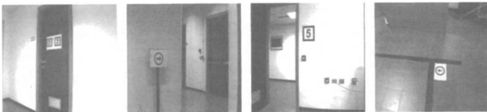
Figure 3. Examples of location of markers and traffic signs in the environment. From left to right: marker located on the doorway; traffic sign located on a pole; marker located on the wall; marker located on the floor on the right side of a track.
