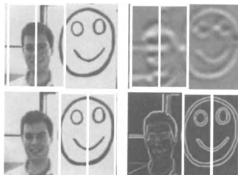
Figure 7. A face vs. smiley. Edge-based methods locate the larger object, which is the flat smiley. Y-Arg detects the three dimensional face, although it is smaller.
